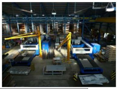
Rods and sheets are temporarily stored in the warehouse and can be cut to size on the company's own machines, in the picture two Trumpf laser cut machines. Alternatively, we can cut sheet metal on two Bystronic water jet machines.
