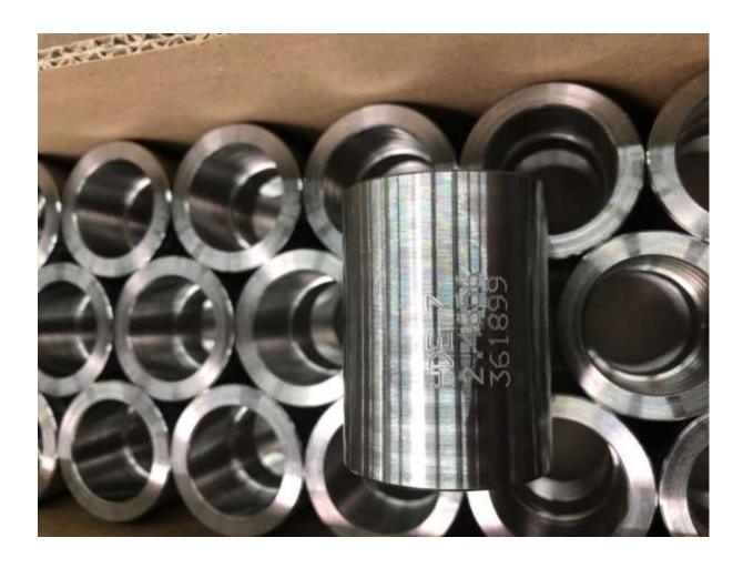
CNC turned/milled welded socket Material 2.4856 made from Round bars with DNVGL Ship Classification. Manufactured by Hempel in Oberhausen.
