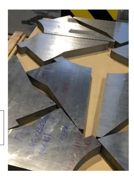
Blanks made of CP-titanium and titanium alloys can be offered on the water jet machines in all possible thicknesses and cutting qualities
